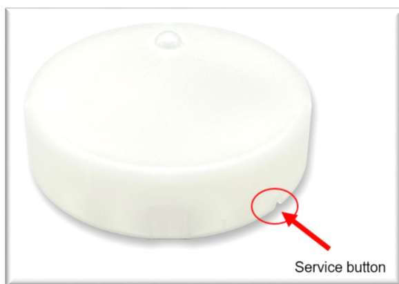
Figure 4: Service button of EnoPuck® CO2 WALL
