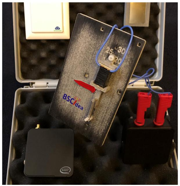
[The BSCiDEA Development Kit contains all components to integrate DEA stack actuators into mechatronic IoT solutions]
