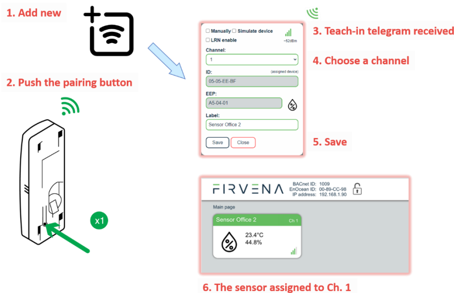
Fig. 6.2 Adding elements – teach-in procedure
