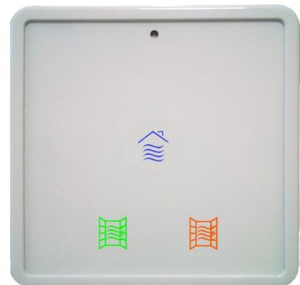
But is window opening really safe? Outdoor air may be polluted and worse than indoor air. Traffic noise can add to the problem. Under such circumstances, the NanoSense IAQ probe can receive air-quality EnOcean telegrams from outdoor air-quality sensors (one per facade) and compare the physiological effects to issue dedicated visual warnings. This warning can also be based on Well V2 outdoor pollution level depending on the setting.
