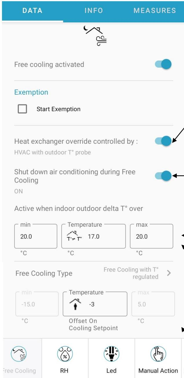
The activation of free cooling generates over ventilation at night when the outdoor air is cooler than the indoor air (without heat exchanger). This freshness accumulates in the mass of the building for the next day.
