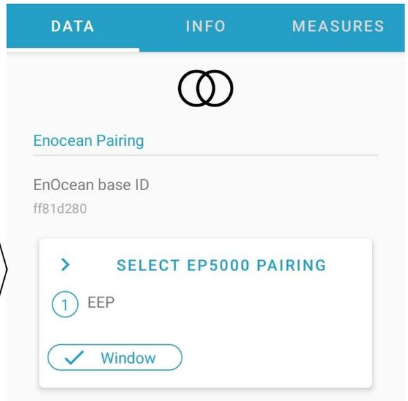
After registering and taping the NFC, the LEDs indicate the pairing process by flashing blue, orange and red in a loop, then the green EnOcean LED lights up indicating that it is waiting for a pairing telegram. After a pairing, the LED will turn off for about 2 seconds and will turn on again if there are still sensors to be paired.
