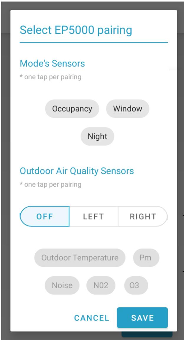
This window is used to select occupancy and night sensors, or even window opening sensors in order to determine an operating **Mode** for the control functions.
