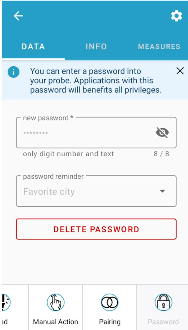
In selecting the Password tab, if the probe has a password already recorded in the smartphone, it is possible de visualize it and also to erase it.
