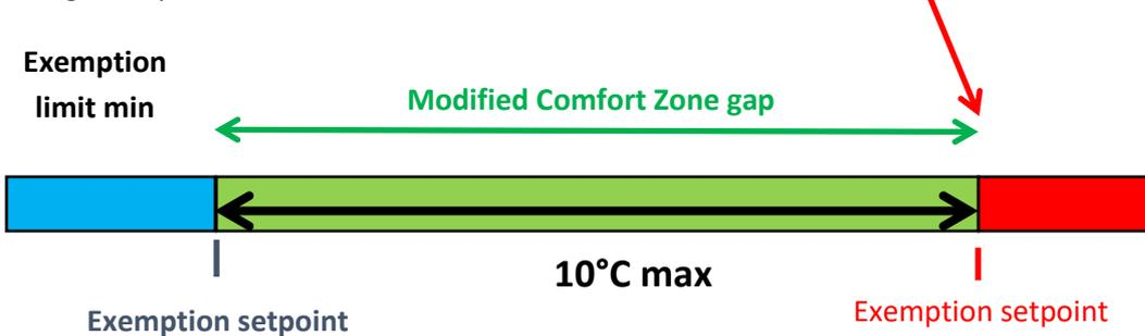
**Attention**, at least 2°C and at most 10°C must be kept between the exemption limit values. (New comfort zone). **The user will have his exemptions limited automatically.**
