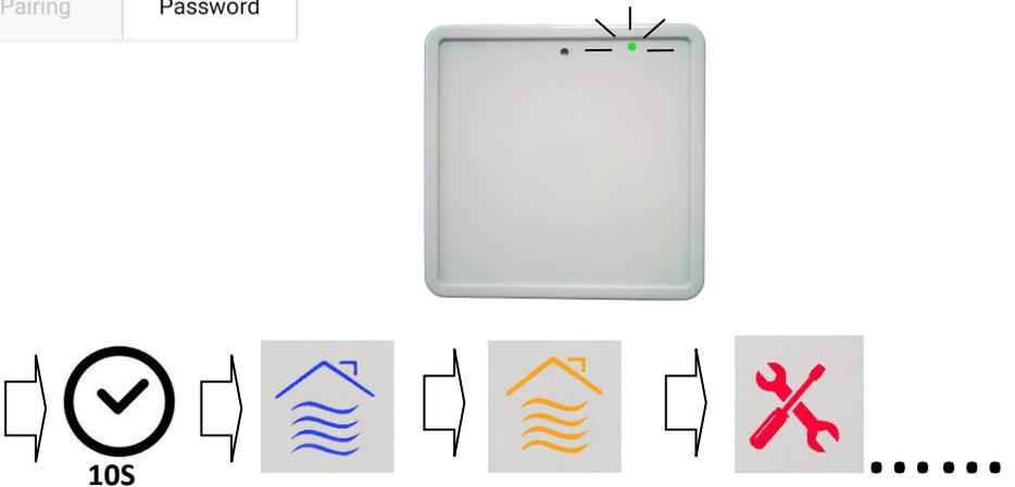
After registering and taping the NFC, the LEDs indicate the pairing process by flashing blue, orange and red in a loop, then the green EnOcean LED lights up each time a pairing telegram is transmitted. Time between pairing telegrams emission is about 2 seconds.
