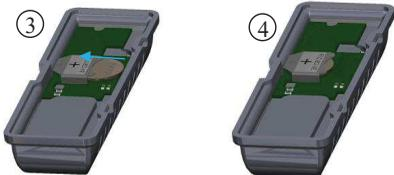
**5.3.2 Replacing the Battery**
