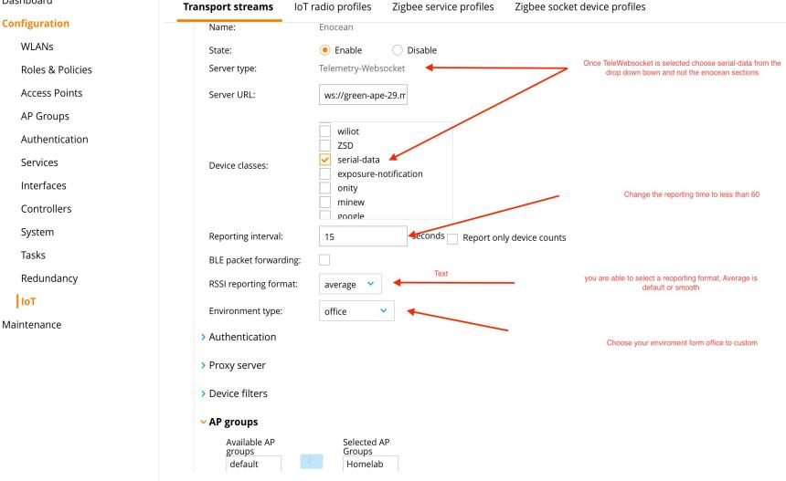
When Telemetry Websocket has been selected a menu box will appear. These are the device options. Select Serial-Data.
