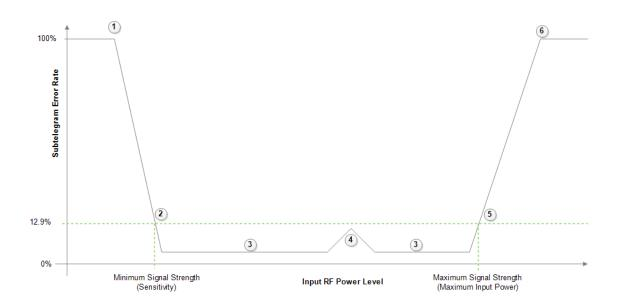
From such a graph, we can determine the characteristics of the receiver, most notably the sensitivity (minimum signal strength at which the subtelegram error rate does not exceed 12.9% - marked as "2" in the diagram) and the maximum input power (maximum signal strength at which the subtelegram error rate does not exceed 12.9%, marked as "5" in this diagram).
