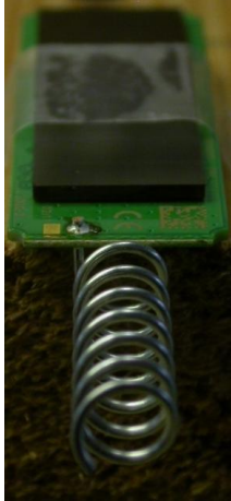
Fig.4 XY-Plane sweep → DUT is mounted horizontally (parallel to earth plane) and turned around its Z-Axis.
