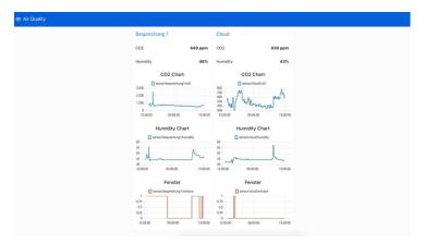
Dashboard for continuous monitoring of carbon dioxide concentration in the ambient air (source: EnOcean GmbH)
