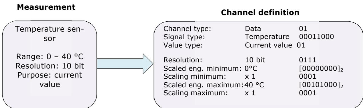
*Example of Data Channel definition: Temperature Sensor*
