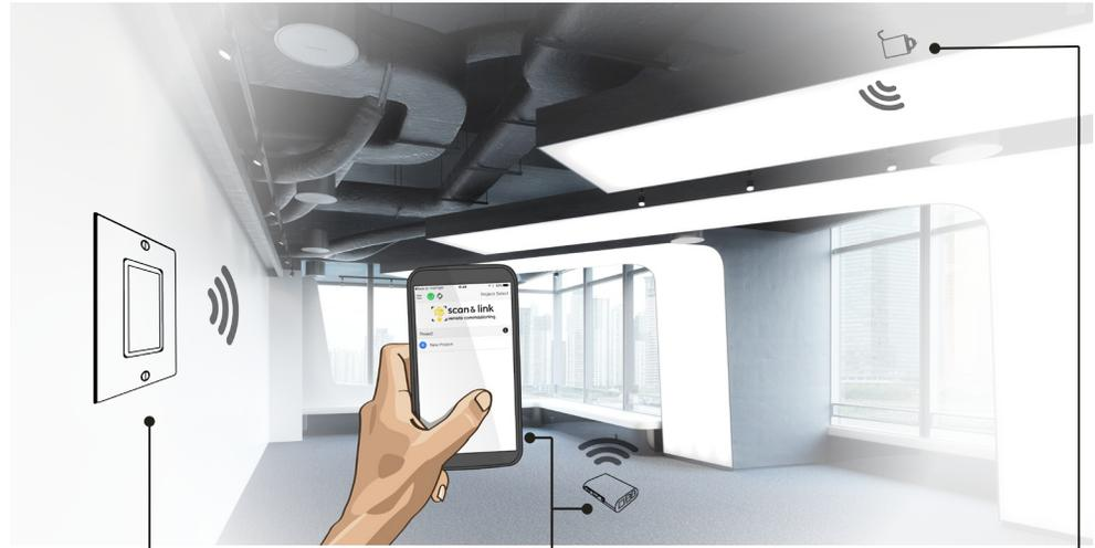
**Wireless sensors and switches** send signals to controllers
