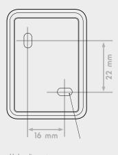
Hole diameter: Ø4 mm ) x2 x2 x2 Wall plugs and screws included
