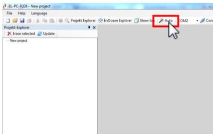
3. The software now tries to connect via the EnOcean USB-stick to the BL-201. Depending on the number of already connected DALI devices, it may take up to approx. 30 seconds until this procedure is finished.
