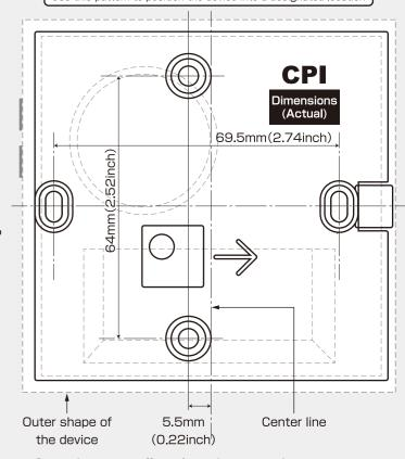
Screw holes are off set from the center line by 5.5mm(0.22inch).
