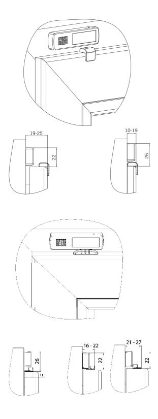
If the sash overlap height is bigger than 19 mm (which is frequently the case with PVC-U and timber windows), the magnet and the wireless contact should be mounted in a way that the magnet is positioned in front of the wireless contact (first illustration).
