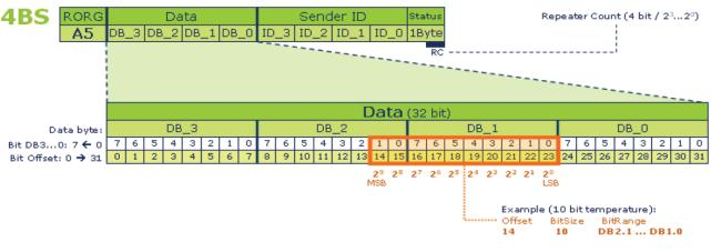
MSB – most significant bit LSB – least significant bit
