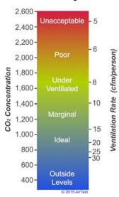
of the solar panel will flash in sequence to indicate the actual  $CO_2$  reading (green=500 ppm, amber=100 ppm, red=25 ppm). The LEDs will also flash every 15 seconds to confirm that the sensor is operating and indicate the general level of  $CO_2$  in the space (green flash = under 1,100 ppm, amber flash = 1,000 to 1500 ppm, red flash = >1,500 ppm). Refer to the chart to see the general meaning of various  $CO_2$  levels.
