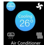
After choosing the device Air Conditioner, long press the button C/D key to adjust the temperature, and the same operation is applied to the floor heating and fresh air.
