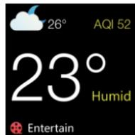
Normally the panel screen is dark, but the backlight will automatically turn on when users get close to it, and the standby interface will be shown on the screen. When user touches any button, the interface will show the latest time operation, and the backlight will be enhanced.
