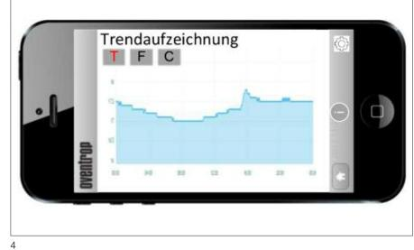
The user interface of the communication centre "Synet CR" allows an easy operation of the whole system via smartphone, tablet or PC. This is a (terminal) neutral WEB App. The user interface is displayed on all terminals in the same manner.
