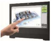
The Linux operating system is installed as well as the Wireless Building Visualization and Control Software. The wireless antenna module is integrated, a power supply is included. The server is locked for other applications. The power consumption is only 11 or 13 watts. For power supply a switching power supply unit 230V/12V DC is included. The 12V cables can be used for permanent connection to a switching power supply unit in a box with wall outlet.
