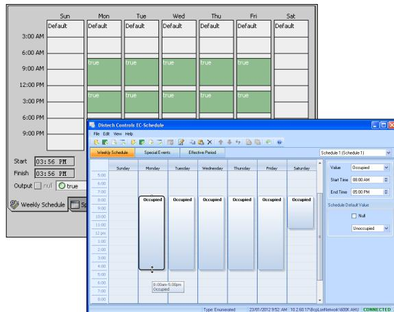
Configure the controller's built-in schedules and holidays from EC-Net<sup>AX</sup> solution (ECB and ECL series controllers), LNS (ECL series controllers), or directly from within EC-gfxProgram (ECB and ECL series controllers) with an easy-to-use point, drag, and click interface. It features a weekly schedule for regular, repeating, events by "time-of-day" and "day-of-week", while a holiday schedule is available to define events for specific days.
