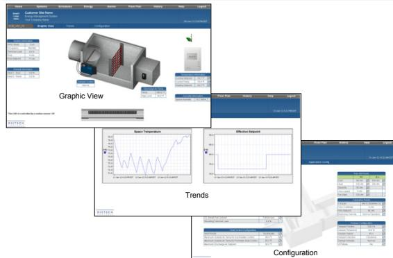
In the EC-Net<sup>AX</sup> solution, dc gfxApplications provide ready-to-use Px graphics pages for the ECL-VAV series of factory preloaded controllers. Once the controller is online, select any one of the standard VAV pre-configured controller applications to use. This provides a proven energy-efficient sequence of operation without any need for programming.
