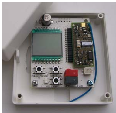
Fig. 3: KNX/EnOcean gateway KNX/ENO 622 from Weinzierl
