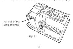
For the best range performance a minimum distance of 1 to 2 cm, should be allowed from the whole length of the antenna to any conductive objects. In particular, the far end of the whip aerial should be mounted as far away as possible from all metal parts. Please note that large metallic or conductive objects between the transmitter and the receiver could cause blocking of the radio waves such that it might result in a range reduction.
