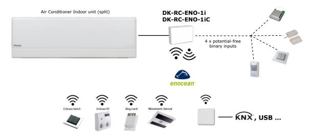
IntesisBox<sup>®</sup> DK-RC-ENO-1i allows monitoring and control, fully bi-directionally, all the functioning parameters of DAIKIN Air Conditioners from EnOcean installations.
