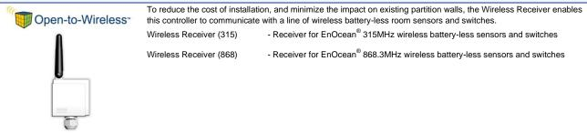
Note that controllers have one wireless port to support a single Wireless Receiver.
