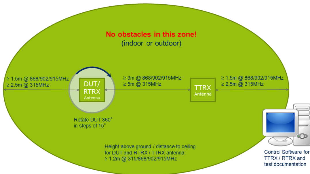
Fig.1 General test site arrangement for a TTRX with an omni-directional antenna
