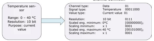
Example of Data Channel definition: Temperature Sensor
